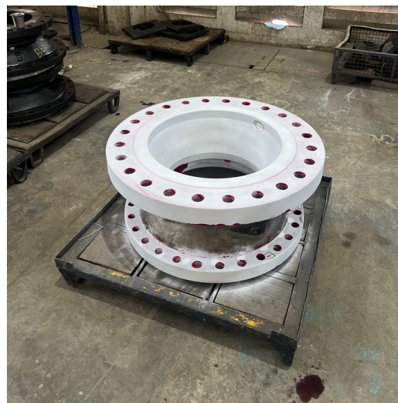
Picture showing the quality testing using paint dye penetration
